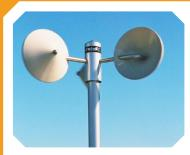
Wind speed is measured with an instrument called an anemometer.
